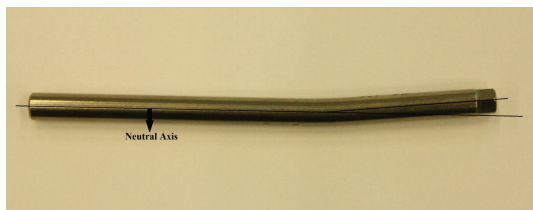
FIGURE 8: Rod failure in flexion moment test.
