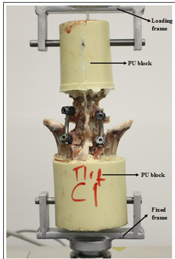
**Figure 2.** Axial compression test set-up.
