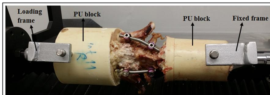
Figure 4. Torsion test set-up.
