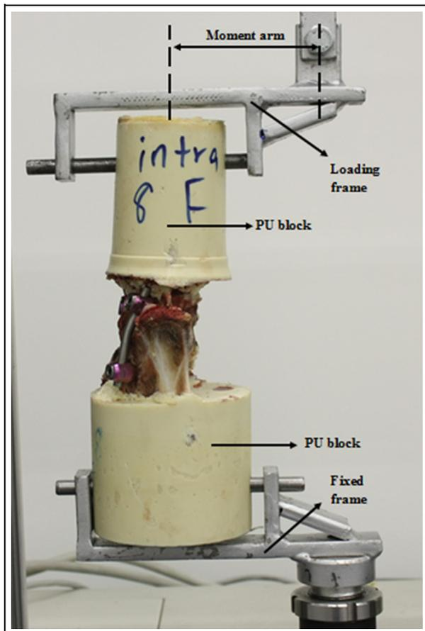
Figure 3. Flexion test set-up.
